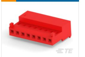
TE Part # CAT-104MTA-NGPMR Nylon Gold Plated Receptacle: 2.54 mm, with Mating Alignment, MTA 100
